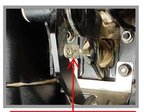
You can make small adjustments to the brake pedal position/pressure by making adjustments to the yoke at the back of the brake pedal arm.
